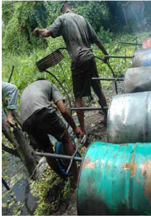
Copper coils attached to the barrels for cooling.
