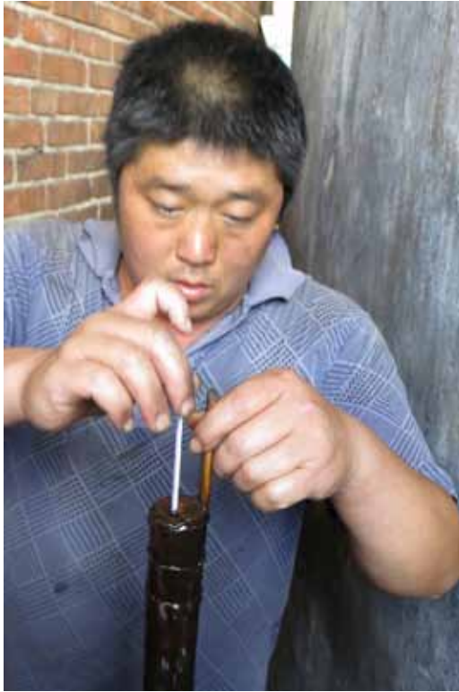
Testing alcohol for ABV with hydrometer.
