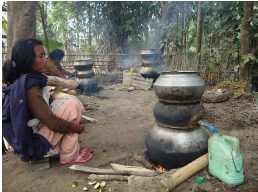
Distillation at a community festival in Dimoria area, Assam. The bottom container contains rice, the middle is for distillation, and the top contains water.
